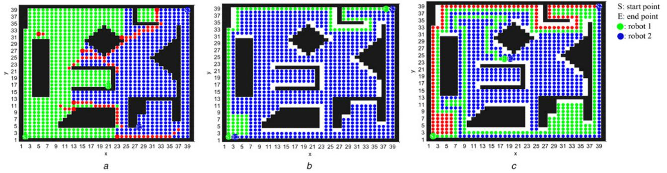
**Fig. 11** Coverage paths using the proposed method and two versions of MSTC in multi-robot systems. The red points are the revisited points
