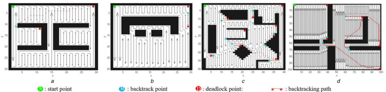
Fig. 7 Experiment scenes. The back area shows the obstacles, the line with arrowheads represents the coverage paths which calculated by the proposed method. Green point is the start point, blue points are backtracking point, red points are deadlock points, right lines are the backtracking paths. There are four scenes
