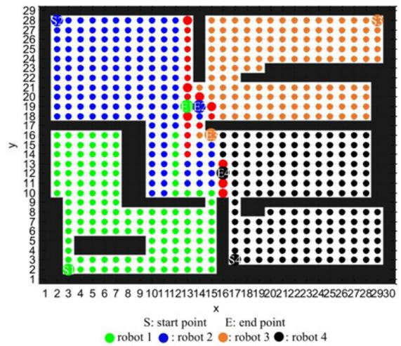
**Fig. 10** Coverage paths performed by the proposed method with four robots. The red points are the revisited points
