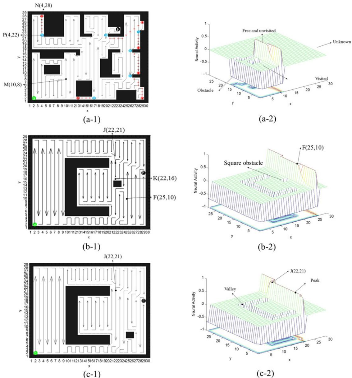
**Fig. 8** Complete coverage path and its neural activity landscapes in the robot current position
