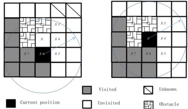
**Fig. 4** Illustration of backtracking list updating
