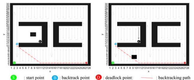
**Fig. 9** Path using the proposed method in unknown environments with a non-stationary obstacle. Left: The path before detecting the squared obstacle. Right: The path after updating the costs
