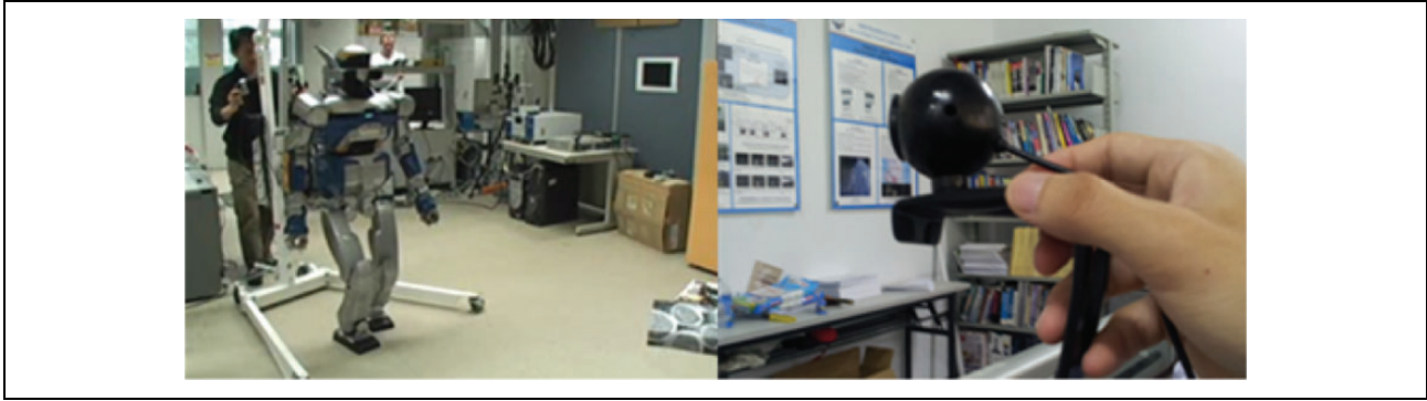
Figure 1. The robot (left) and handheld camera (right) are recognizing the environment and localizing themselves using visual SLAM algorithm. SLAM: simultaneous localization and mapping.
