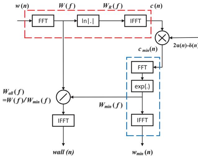
Fig. 2. Decomposition of minimum phase component and all-pass component using homomorphic filtering.
