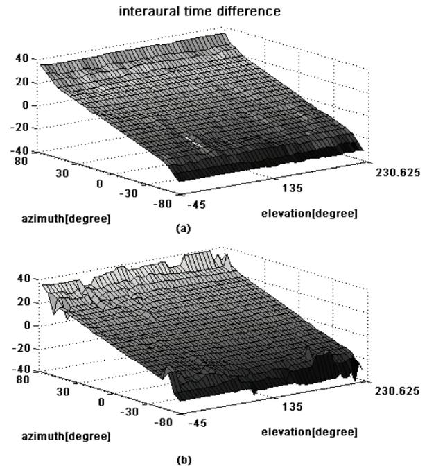
Fig. 3. Comparisons for ITD. Up: obtained by our proposed method. Down: attained by GCC-PHAT.
