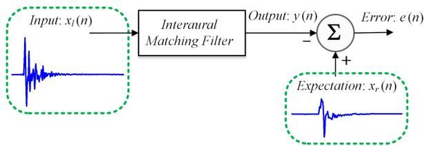
Fig. 1. Linear discrete time Interaural Matching Filter. Taking  $x_l(n)$  as the input of IMF and  $x_r(n)$  as the expectation is equivalent to the contrast situation in theory.
