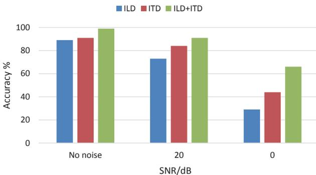
Fig. 5. Comparing the azimuth localization accuracy of ILD, ITD and joint of ILD and ITD in different SNRs with 5° tolerance.
