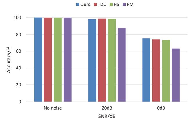
Fig. 7. Comparing localization correct rate using the proposed method and several popular methods when the tolerance is 10°.
