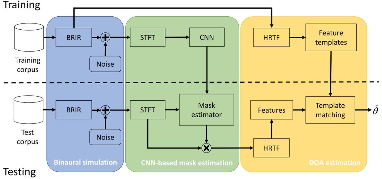
**FIGURE 1** Schematic diagram of proposed head-related transfer function–reserved mask-guided sound source localization method. The upper part is the training phase constructing a convolutional neural network–based mask estimator and the binaural feature templates. The lower part is the test phase to estimate the azimuth through template matching and time-frequency masking.
