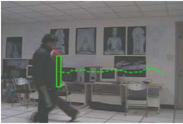
Fig.1. The new definition of temporal neighbor works when occlusion is detected
