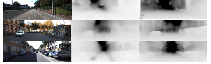
Fig. 2. Single-view depth prediction. The images in the first column are the original input images, and the depth maps in the second column is the results of sfm-learner, while the last column of depth maps are predicted by our method.
