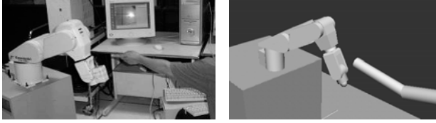
Fig. 2. Manipulator, human arm and their models
