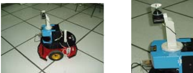
Fig.1 Human motion detection system implemented on Pioneer 2-Dxe robot
